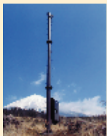
Volcano monitoring camera using optical fiber network
